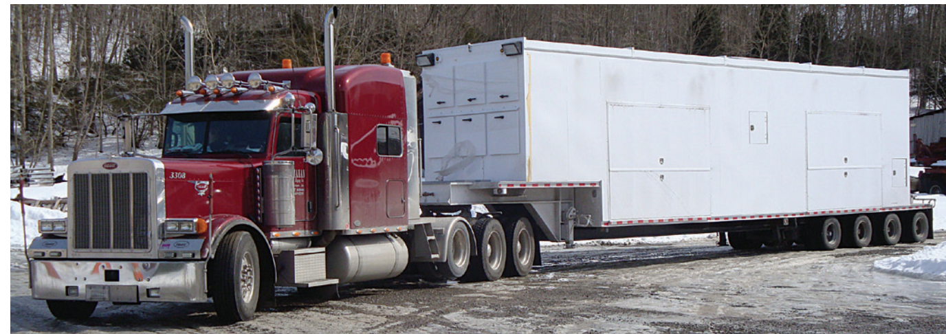
230kV Enclosed Mobile Substation
